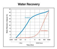
Fast and thorough water separation results in rapid beaching, creating a faster drying load-bearing structure that is ready more rapidly for the next lift. Fines are incorporated into a solids matrix that maintains structural integrity. You get a drivable
