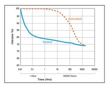
The numbers are remarkable. Laboratory testing shows a mere 15 minutes required to produce 21% as supernatant, versus 200 hours with untreated underflow.
